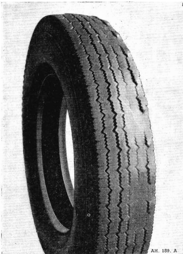
Fig. N.16. Irregular 'Spotty' wear, to which a variety of causes may contribute.
