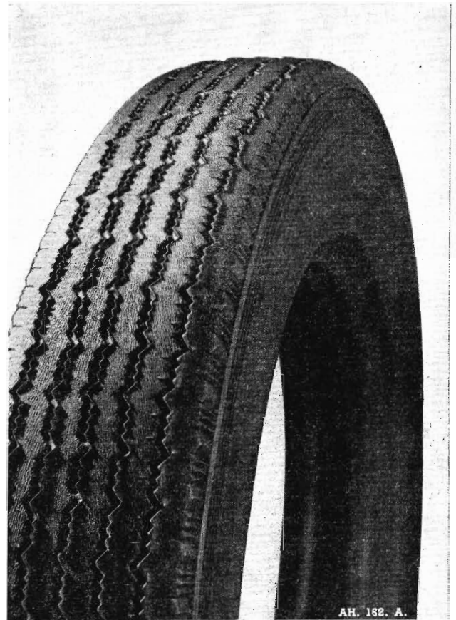
Fig. N.17. Fins or feathers caused by severe misalignment. With minor misalignment, probably aggravated by road camber, the ribs may have sharp edges instead of upstanding fins. The conditions will usually be accompanied by heel and toe wear across the tread due to its being distorted and worn away laterally instead of in a true rolling direction.
